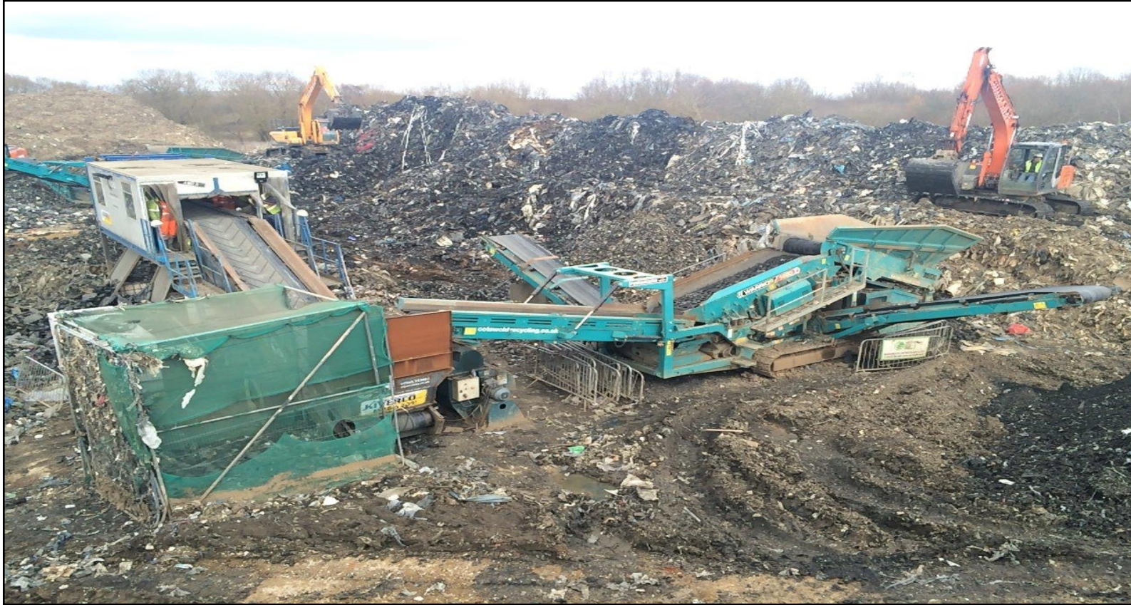
Segregation of waste streams comprising screens, blowers and picking stations.
